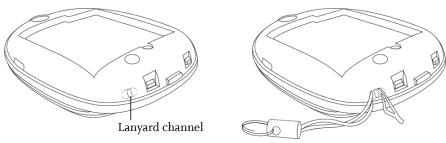
Replace the battery cover, making sure the lanyard strap feeds out the cover's notch next to the battery latch.
